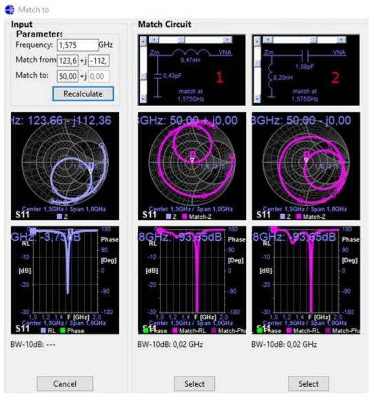
Matching filter 1 is a Low-pass LC filter, and filter 2 is a high pass LC filter.
