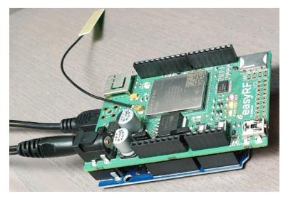
Verify the Arduino board is recognized by the PC/Laptop, and upload an example of your choosing to the Arduino board. When opening the COM port in the Arduino software, make sure to put it on 9600 baud.
