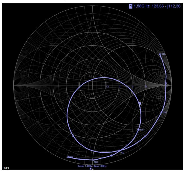
The matching filter can be calculated by hand, or the "Match Circuit" feature can be used. The Match circuit feature Is a special tool made by the manufacturer and is integrated in the VNA software.
