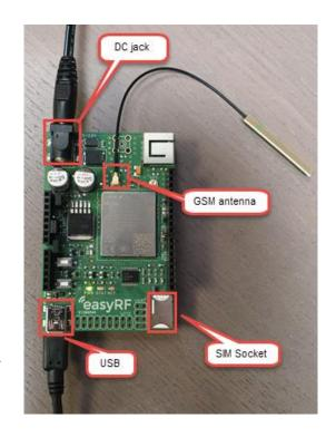
When above steps are followed, the shield is ready to receive AT-commands. Before a serial connection to the shield can be opened, the correct drivers need to be installed on your device.
