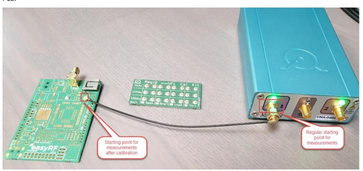
The VNA measurement will return 3 graphs, the Impedance, the return loss and the forward loss of the antenna circuit. These 3 graphs are used to interpret the total performance of the antenna circuit. Since the measured antenna is a GNSS antenna the optimal performance should be at 1575 MHz.
