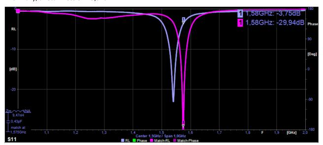
After matching the impedance the overall performance of the antenna circuit will be greatly improved.
